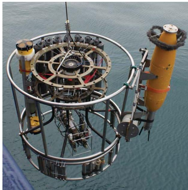
*Multichannel microstructure profiler "Baklan" attached to a rosette sampler for studying mixing processes. At a depth the profiler gets detached from a rosette sampler and takes measurements while free falling*
