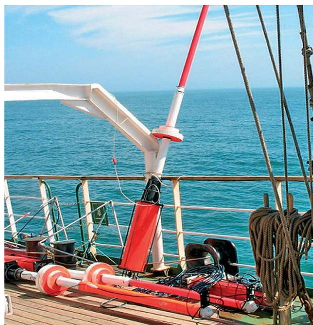
Autonomous Hydroacoustic Buoy with satellite connection to the Internet
