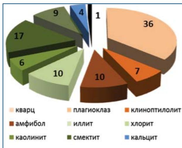
Mineral composition of aerosols in the surface layer of the transatlantic section, April 2015 (diffractometer)
