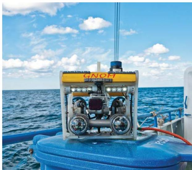
*Gnom PRO (works at depths up to 300 m) is equipped with an all-round sonar and digital camera*
