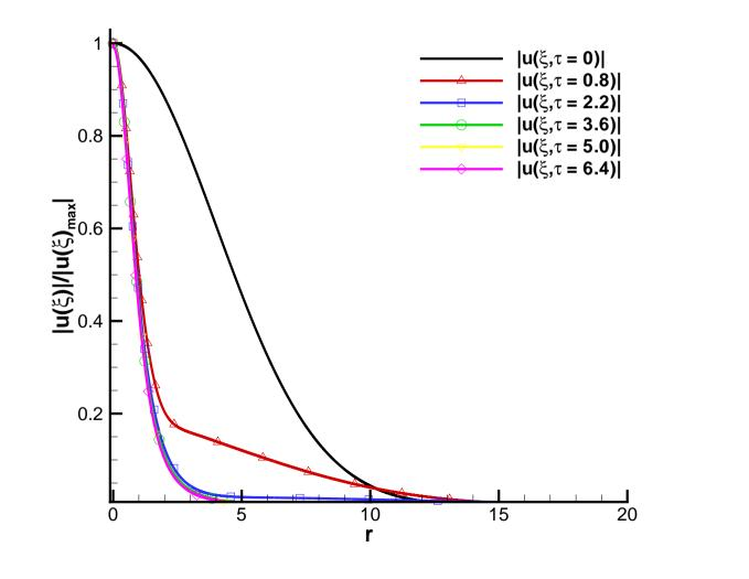
The formation of the eigen mode for l = 1: dependences of  $|u_1|$  normalized by its maximum amplitude at different times.
