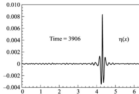
Fig.5. Typical profile of breather
