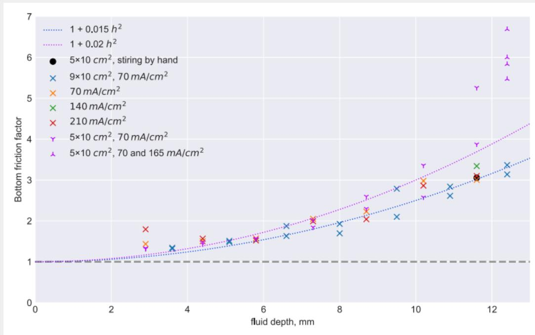
$$\text{Bottom friction factor} = \frac{\alpha_{exp}}{\alpha_0} \quad \alpha_0 = \frac{\pi^2}{4} \frac{\nu}{h^2}$$
